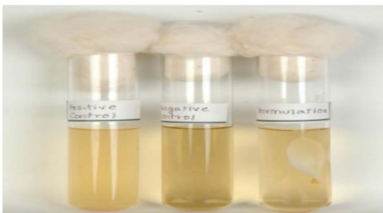
Figure 5: Observation of Sterility test done in Soya bean Casein Digest medium (SCDM)
